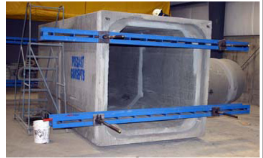
Typical restraining fixture, utilizing steel beams and high tensile-strength threaded retaining rods.
