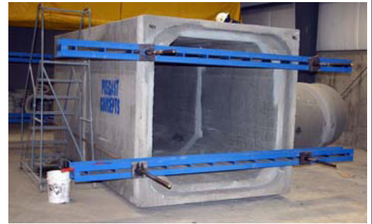
Typical restraining fixture, utilising steel-channel retaining beams and high tensile-strength threaded retaining rods.
